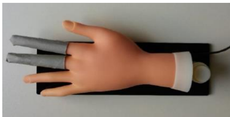
Figure 10. EDA simulator in human hand form with active electrodes on index and middle finger. Taken from (Geršak, 2020)
